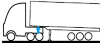
Drive carefully towards the trailer until the kingpin bolts in the locking device of the fifth wheel on the truck.
