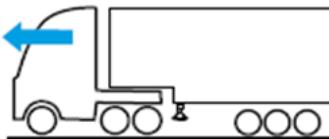
Connect the couplings, hoses and electricity. Next turn or lift the parking legs.
