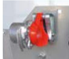
Suspend brake hoses after disconnection. Thus, it prevents possible sand / pollution that can enter the EBS modulator by means of compressed air lines.
