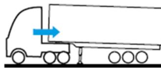
Lift the trailer so that the parking legs are 5 cm clear off the ground.
