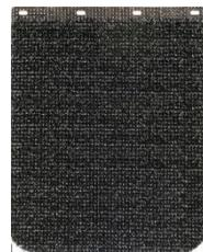
The anti-spray mats of the mudguards must be cleaned on a regular basis with a high pressure washer.
